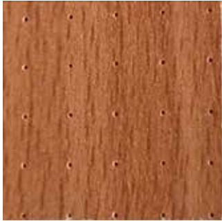
MELAMINIUM WOODENWOOD PANEL B; S2;do / WOODEN PAINTED TH. 14 MM. HOLE D.0,5 MM. PITCH 6X6 MM. BLACK SOUND-ABSORBING FABRIC IN THE BACK
