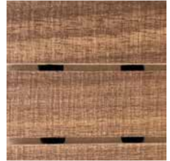
MELAMINIUM WOODENWOOD PANEL B; S2;do / WOODEN PAINTED TH. 14 MM. REAR HOLES PITCH 32 X 32 MILLING PITCH 32-3. BLACK SOUND-ABSORBING FABRIC IN THE BACK
